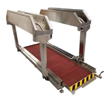
For high throughput food production and processing facilities, PROTECH XV sanitizes hands, gloved hands, and street shoes to full rubber boots on a continous walk through system. The system automatically sprays proprietary E3 sanitizer in the hand troughs and replenishes the footwear sanitizing pan with additional hard surface sanitizer to keep the PPM at a high, consistent level.
